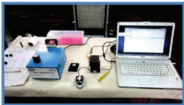
Avalanche photodiode based bioluminometer developed in the Institute
