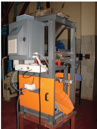
Servo-based automatic grain weigher for flour mill
