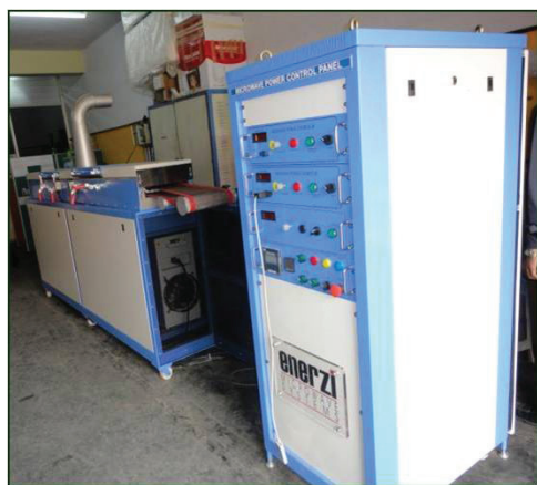
Custom-made Microwave dryer for continuous operations
